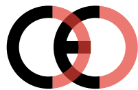
False CE Mark (too close)
