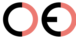
False CE Mark (too far)
